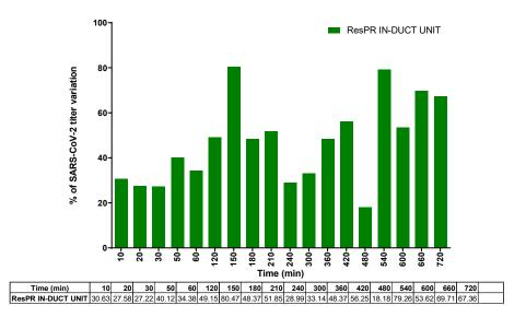
Figure 2. Reduction (%) of SARS-CoV-2 mean titer in relation to control samples of the inoculum collected at 18 time points (from 10 to 720 minutes) from 24mm x 24mm aluminum foil pieces exposed to a ReSPR IN-DUCT device.
